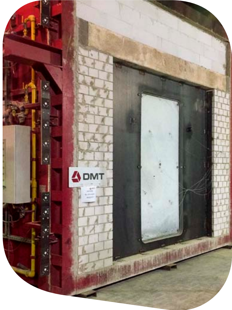
Testing of a ship bulkhead with Pilkington Pyrodur ® TM: Besides fire safety, there are increased requirements for the system glazing.
