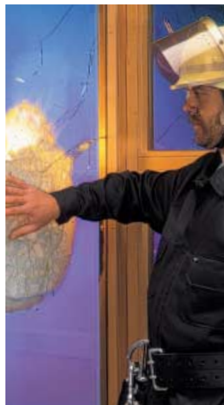
Glass intumescence as shown above applies to Pilkington Pyrostop ™ and Pilkington Pyrodur ™ .
