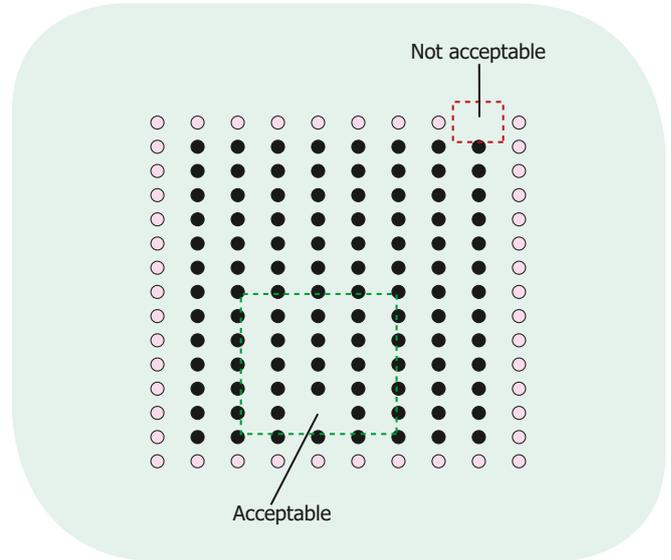
The microspacer grid ensures that the two glass panes are kept a fixed distance apart. When looking through the window from a distance of 2-3 m they become imperceptible.
