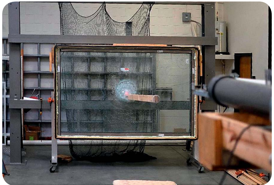
Missile impact tests with hurricane-rated fire-rated Pilkington Pyrostop® glass at Underwriters Laboratories® (UL) in Northbrook, Illinois: the wood "missile" shot at the glass at 56 km/h (34 mph) simulates the impact of large wind-borne debris. Photo: TGP
