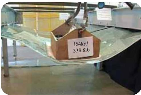
**Planar™** | SentryGlas® Plus System Panels undergoing load testing
