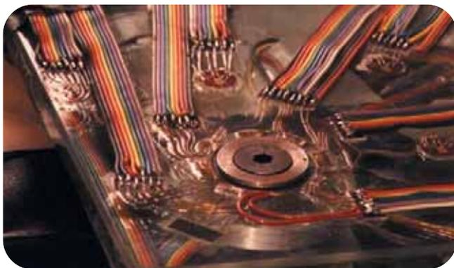
Strain Gauge Testing around Pilkington **Planar™** countersunk hole.
