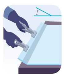
Score the glass as before and run along the cut with glass pliers. Use a suitable hand tool to assist in gripping the glass when snapping out.
