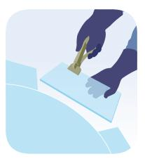
"V" notches are cut and the exposed wires scored with a blade. The strips are then removed separately.
