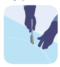
A template is placed under the glass and the shape traced with a cutting wheel.
