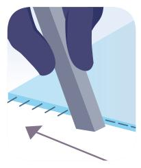
The protruding short wires can be folded over flush by running a metal tool or special roller tool down the edge of the glass.
