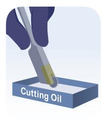
Score in a continuous and uniform depth using a cutting wheel lubricated with cutting oil. Run the cut along the score by flexing the plate by hand or with glass pliers.
