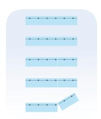
You may find that the position of the wire within the glass is closer to one face of the glass than the other. Flexing the glass where the distance between the wire and the glass face is least, may help reduce the risk of edge crush.
