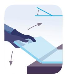
Weaken the wires by carefully moving the cut plate alternately up and down in a controlled manner to avoid damage to the top and bottom edge surfaces.
