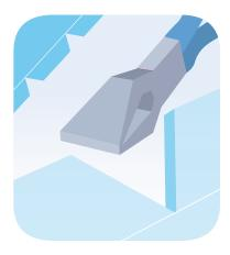
First, score as before, then separate into sections by cutting "V" notches out of the strip.
