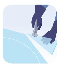
Excess glass is removed within an inch or so of the cut.
