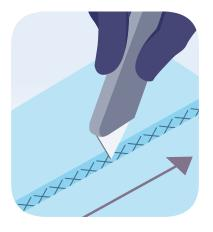
Cutting techniques are basically as before but the surface of the exposed wires should be scored with a sharp blade before snapping out.
