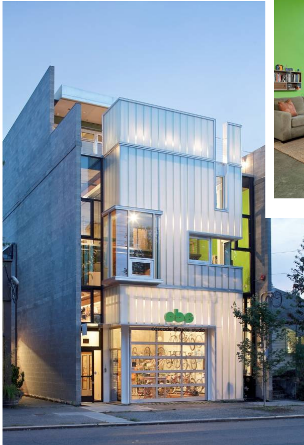
Pilkington Profilit™ K25/60/7 T-H with TIM (translucent insulation material)
