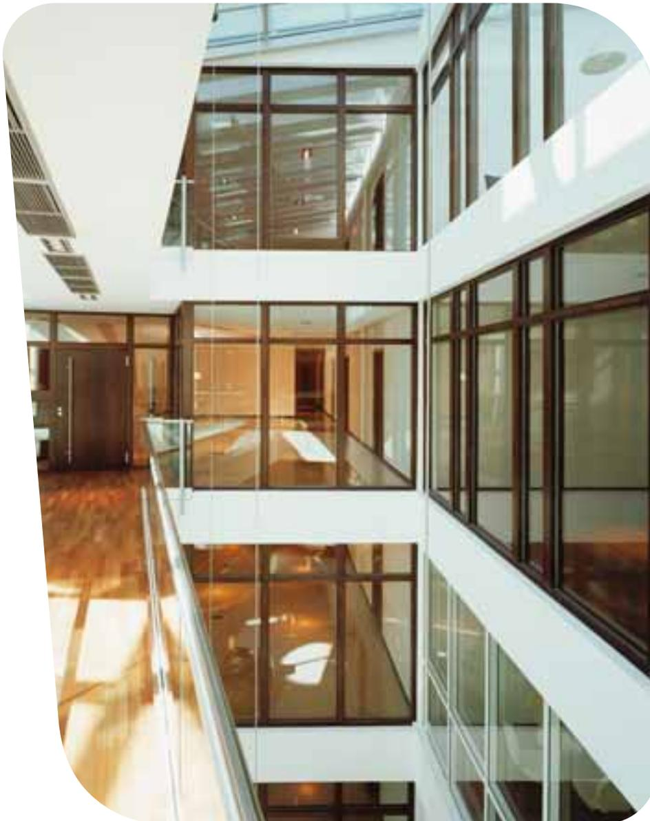
In the entrance lobby, which is bathed in light, 12-metre long crosspieces are arranged at an angle to the building axis to link the separate parts of the building. Both ends of the crosspieces are connected to the building sections which use class F(EI) 90 glass for their windows and doorways.
