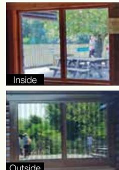
Although invisible to human eye, many species of birds are able to detect UV patterns on the glass surface to avoid collision.
