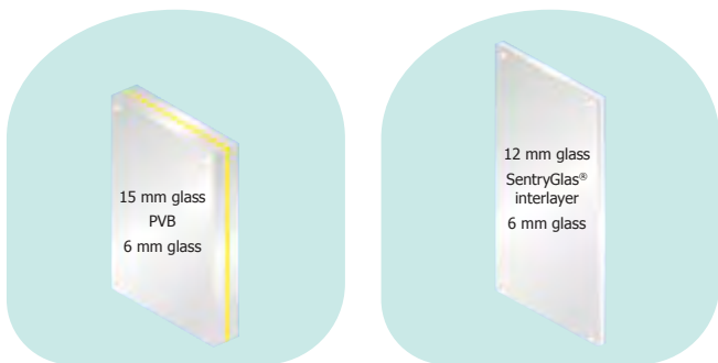
Figure 8.1. Performance comparison of Pilkington Planar ™ using SentryGlas® versus PVB interlayers.
